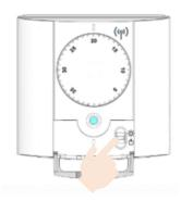
8. The pairing can be tested by turning up the temperature on the room thermostat. The paired Channel on the master (in this example channel 3) will switch on and lights up red. The pump is switch on after approx. 1 minute and lights up green.
