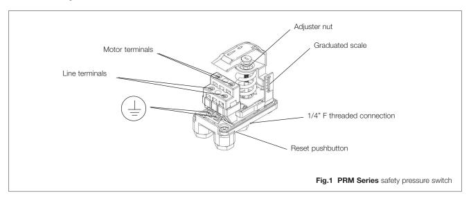
The **PRMIN Series** pressure switch has two normally open electrical contacts, which are insulated from each other. When the system is pressurised the contacts close. When the minimum shut-off pressure setting is reached, both contacts **open**. To adjust the shut-off pressure, if necessary, turn the adjuster nut. The set value is shown on the graduated scale.
