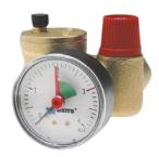
Safety unit for closed circuit systems according to EN 12828, up to 50kW complete with insulation - compact version, brass body with built-in air vent and safety valves incorporated into casting. Pressure gauge (0÷4 bar).
