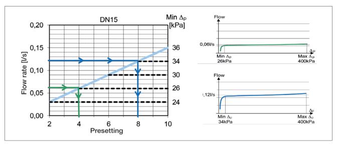
The flow regulating group has the authority on all its full linear stroke. By using a modulating actuator, this allows to maintain proportionality between the control signal and the actual output flow (example for a WATTS actuator with control signal 0-10V type EMUJC). In the example above, for a maximum flow of 0,12l/s a presetting of 8 is determined on a DN15 valve. The valve will start to operate at a  $\Delta p$  of 34kPa.
