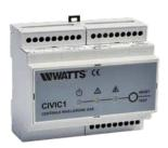
Gas detector control unit for connecting 1 **UR13 or UR21S Series** sensor; with LED-based optical interface (power ON, fault, gas alarm) and internal buzzer-based acoustic interface. Control output for gas alarm and OC output for fault indication. In self-extinguishing plastic housing, for DIN-rail mounting.
