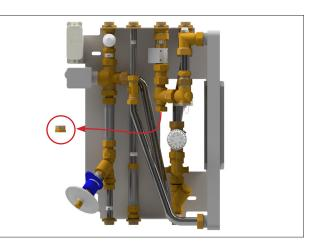
2. Install the water hammer arrestor.
