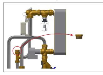
2. Install the water hammer arrestor.
