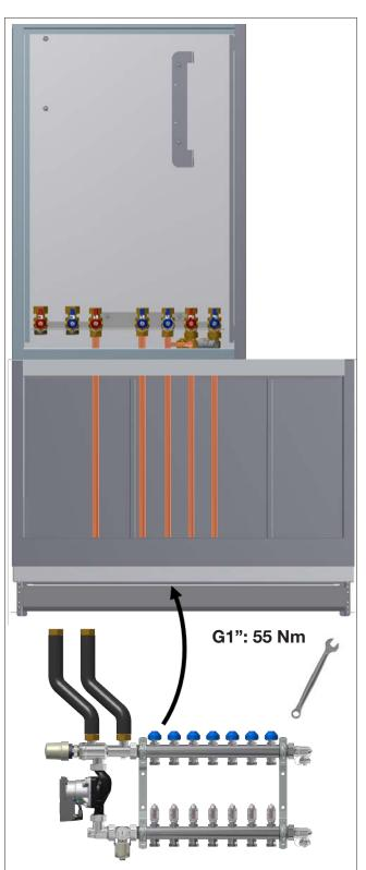
7. Insert the HIU 2 Heat Interface Unit the cabinet and connect it to the connecting rail (for further details, refer to the HIU 2 instructions).
