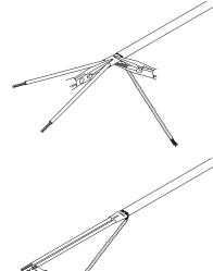
Pull both conductors outwards and squeeze the heat-shrink sleeve. If no adhesive appears re-heat and re-squeeze.
