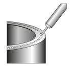
Carefully turn the lid clockwise. Do not damage the black gasket between body and top part.
