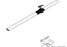
Unconnected heating cable end sealing Score and remove the jacket sleeving over
