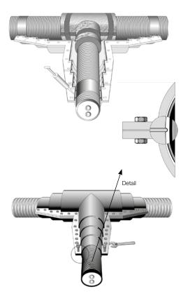
Apply the sealant uniformly to the grooves of both shell-shaped casings. We recommend a thickness of about 4mm and a width of 5mm.
