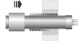
Push the Microflex pipe through the bricked in corrugated casing.
