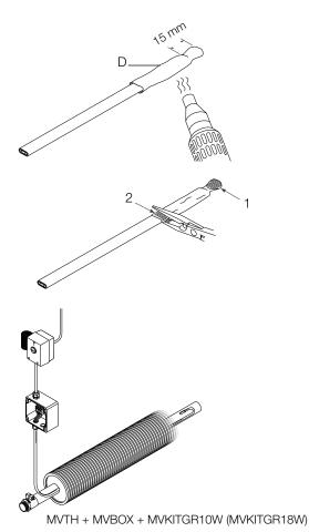
Place heat-shrink sleeve (D) over braid (leave 15mm sticking out) and shrink with heat source. Proceed immediately to the next step.
