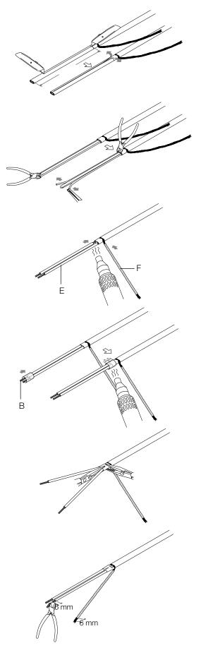
Score with a sharp utility knife and remove the electrical insulation over a length of 150mm. Take care not to damage the conductors.
