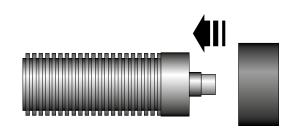
Slide a shrink sleeve (MHM model) over the casing prior to positioning the Microflex pipe in the inspection chamber.
