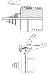
Put the rubber end-cap over the carrier pipe and push it against the insulation. If needed, wet the carrier pipe with water. Do not use soap, grease or oil for lubrication.
