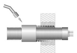
Use a heat gun to gently shrink the sleeve half onto the corrugated pipe and half onto the casing of the Microflex pipe.
