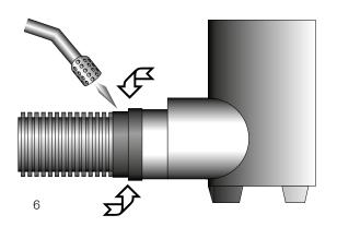
Gently shrink the MHM sleeve onto the casing using a heat gun or mini torch to ensure a waterproof connection between the casing and inspection chamber.
