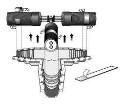
Cut the bitumen strips to suit the pipe casing outer diameter. Remove the protective layer and fit the bitumen strips to the inside of the insulation casings at the pipe entry points.
