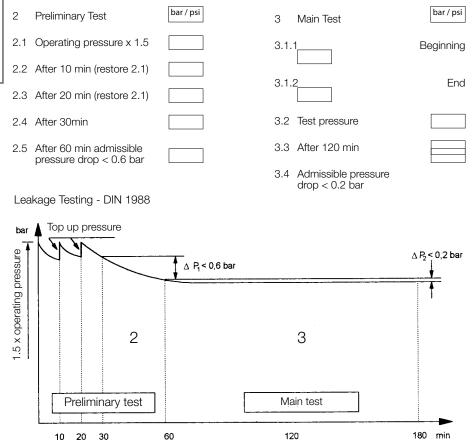
Test the finished pipe-work before concealing! The correct execution and documentation of the pressure test for the entire piping system are requirements for the warranty.
