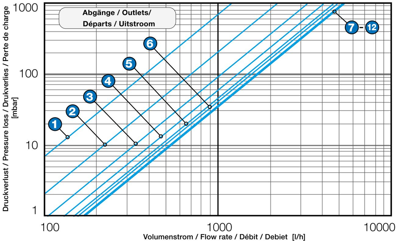
Einstellung des Regulierventils / Adjustment of the control valves
