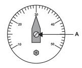
Once the handle is removed, undo screw "B" and the stop "C". Replace the dial 10°/50°C by the 30°/70°C (art. n° 22TB100740U), re-tighten screw "B" and the stop "C", then reposition the handle to face mark 30°C. Re-tighten screw "A". It's done!
